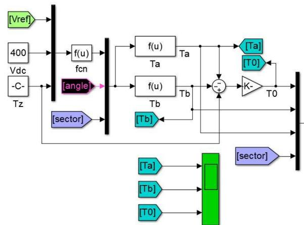
Fig 15. Applying mathematical operations to generate times  $T_0$ ,  $T_1$ ,  $T_2$
