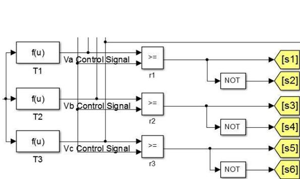
Fig 16. Extracting switching signals S1-S6 using times  $T_1$ ,  $T_2$ ,  $T_3$
