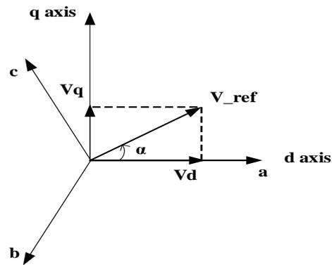
Fig 8. Conceptual relation between reference voltage vector and its angle with axis d
