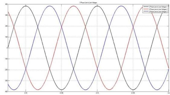
Fig 24. Waveform of output line voltage of virtual inverter sector in indirect matrix converter
