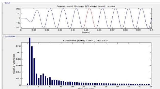
Fig 27. Harmonic spectrum of waveform of output phase voltage in virtual inverter sector of matrix converter
