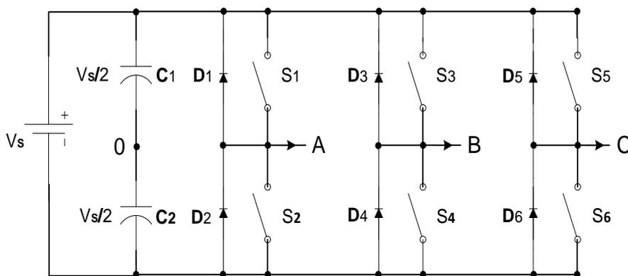
Fig 4. Structure of three-wire three-phase inverter
