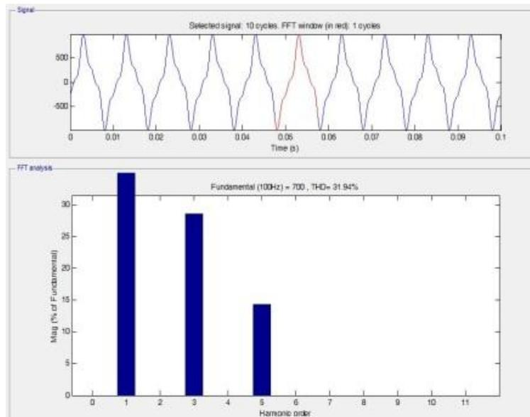
**Fig 19.** Harmonic spectrum of input voltage of matrix converter for phase B
