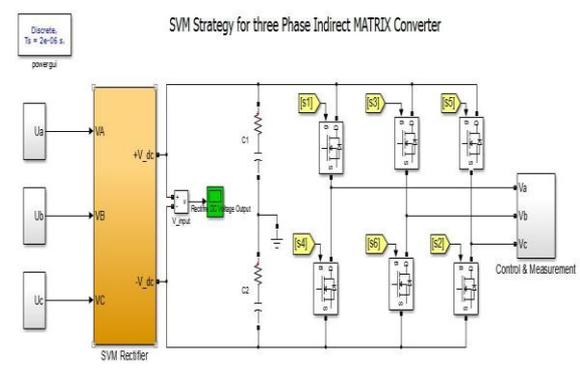
Fig 11. General schema of simulation of indirect matrix converter
