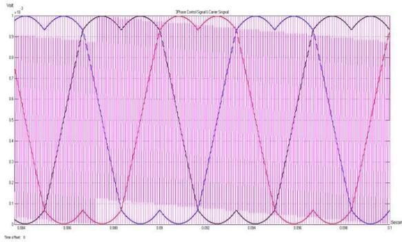
Fig 23. Waveform of inverter control signal along with carrier wave
