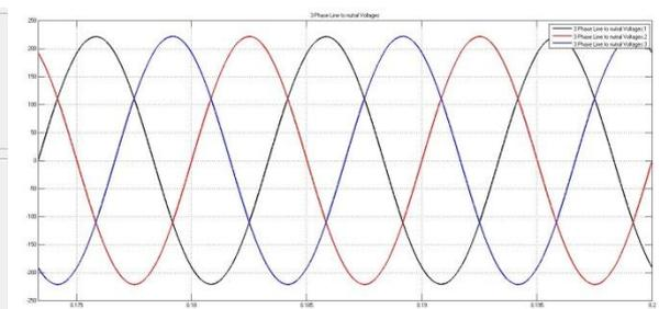
Fig 26. Waveform of output Phase voltage of virtual inverter sector in indirect matrix converter
