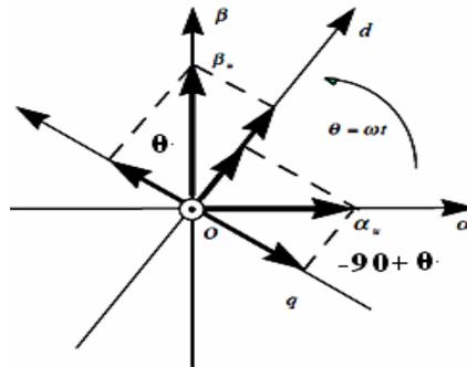
Fig 2. Converting static coordinates of  $\alpha\beta$  to rotating coordinates of dq
