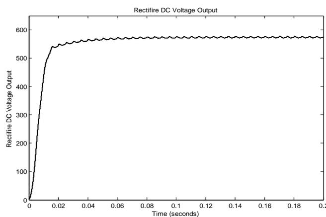
**Fig 21.** Waveform of rectifier output voltage
