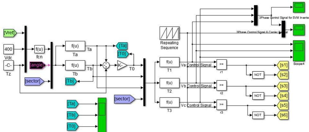
Fig 14. Generating switching signals of inverter sector of indirect matrix converter
