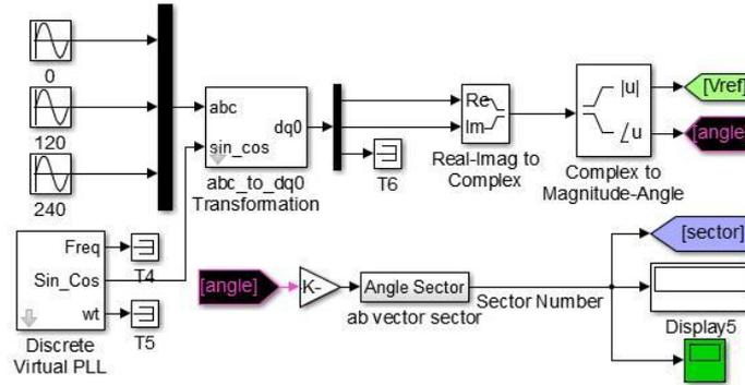
Fig 13. Generation of reference voltage vector along with its displacement angle
