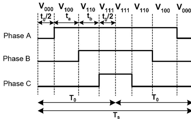
Fig 10. Symmetric switching pattern in SVM method
