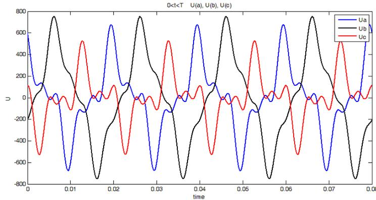
Fig 17. Input wave of indirect matrix converter
