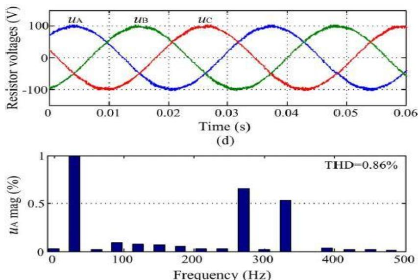
**Fig 28.** Waveform of three-phase output of matrix converter along with its harmonic spectrum
