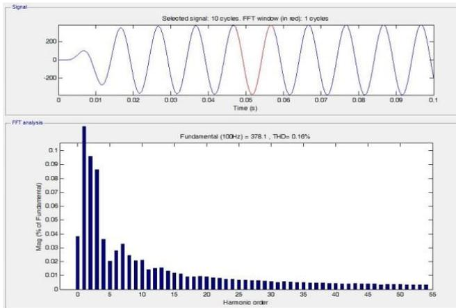
Fig 25. Harmonic spectrum of output line's voltage waveform of virtual inverter sector in matrix converter
