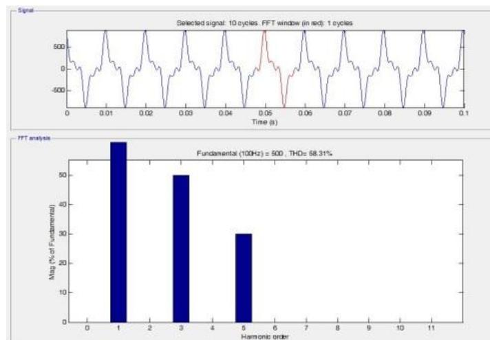
Fig 18. Harmonic spectrum of input voltage of matrix converter for phase A
