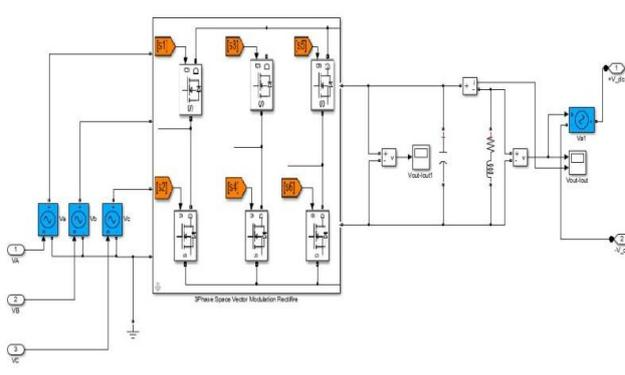
Fig 12. General schema of virtual rectifier sector of 2matrix converter
