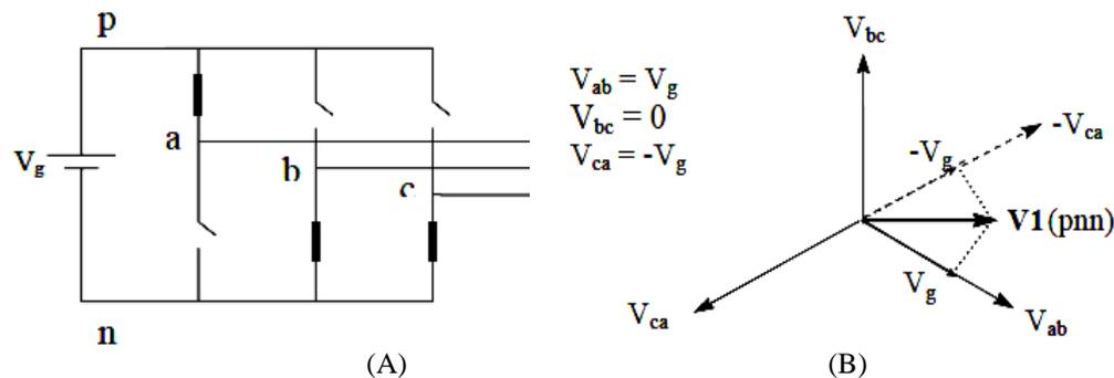
Fig 6. A) Circuit mode of connection (100), B) vector analysis of mode (100) with line voltage vectors
